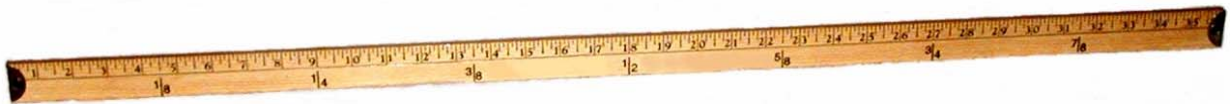
The Yard is the U.S. Customary System and is defined as 0.914 4 meter.
