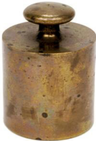
The Avoirdupois pound is the U.S. Customary System and is defined as 0.453 592 37 kilogram.
