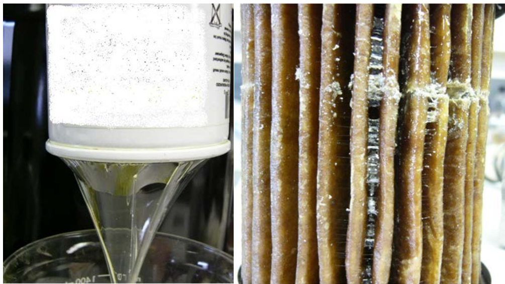
Figure 11: Unsheared DRA (left) and DRA blocking retail filter media (right) 7
