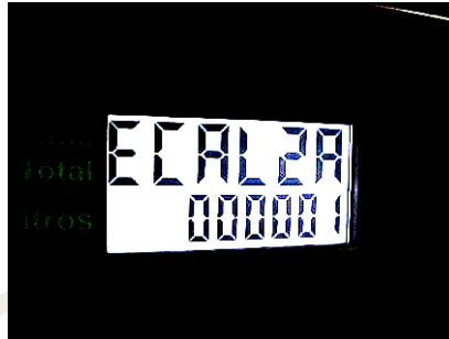
Example of audit trail for side two meter A with one event
